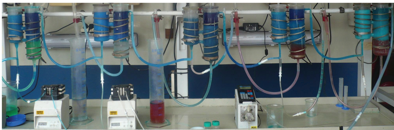
Fig. 1 Operational continuous extraction process for the separation of cobalt from nickel with the trihexyl(tetradecyl)phosphonium chloride ionic liquid (Cyphos ® IL 101) as the extraction phase. The different stages are (from left to right): an extraction stage, a washing stage and three stripping stages in counter-current mode.
