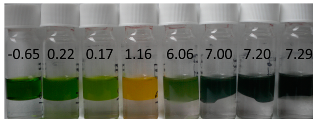
Figure 5. Color switch observed for the IL phase because of the extraction from the transition metal solution at different pH values. pH of the aqueous phase is mentioned on each bottle.
